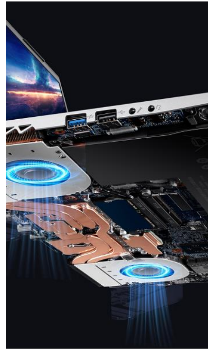
Heat dissipation system with two fans and four copper tubes
